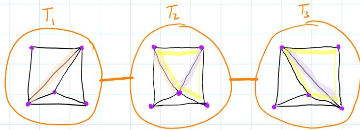
The **FLIP GRAPH** of a point set  $S$  is a graph whose nodes are triangulations of  $S$ . Two nodes  $T_1$  and  $T_2$  are connected by an edge if one diagonal of  $T_1$  can be flipped to obtain  $T_2$ .
