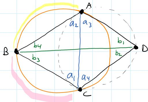
The smallest angle is one of  $\{b_1, b_2, b_3, b_4\}$ , so the triangulation containing  $\overline{AC}$  is fatter, and thus is the Delaunay triangulation.
